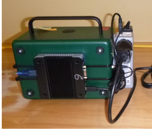
Figure 6. Continuous radon monitor showing a small central processing unit mounted to rear. The power supply for the monitor and computer is shown at the right.
