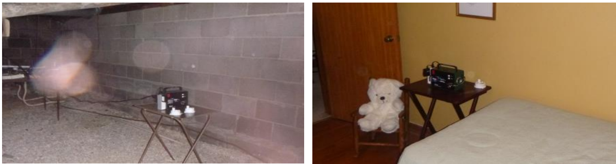
Figure 7. Radon monitoring equipment in place in a crawl space (House 4, left) and in an upstairs bedroom (right)
