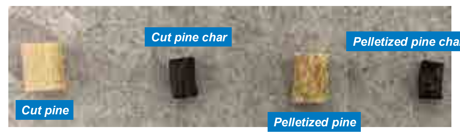
Figure 3. Photograph of cut and pelletized pine and char samples characterized in this study
