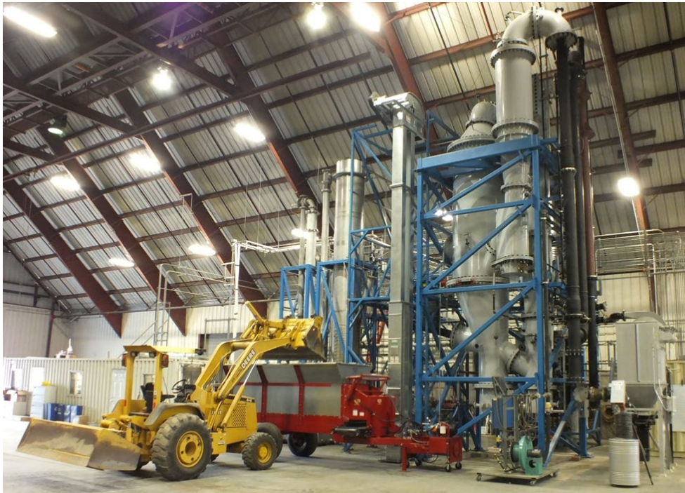
1MWth, 5 tons of dry biomass per day
